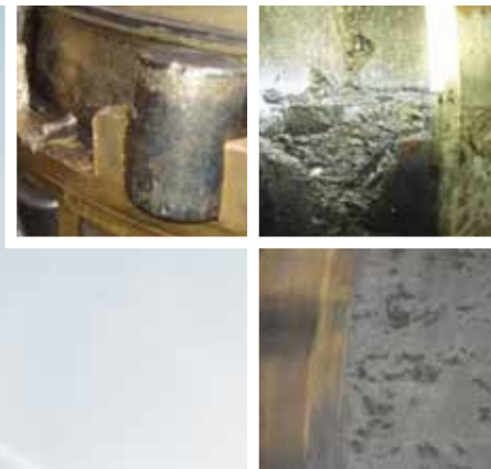
Pictured above is damage seen in the field on spherical roller bearings used in three-point mount turbines.
